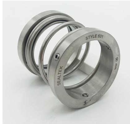
Rotary pusher type mechanical seal with cylindrical heavy duty spring. The open design of the spring avoids accumulation of solids, the flexible drive tolerates shaft misalignment and keeps always faces contact without driving pins. Available in balanced design.
